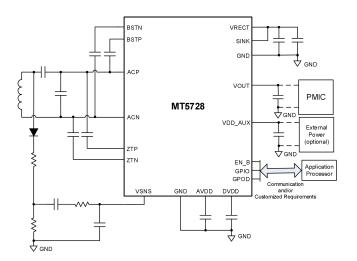
**Figure 1 Typical Application Circuit**
